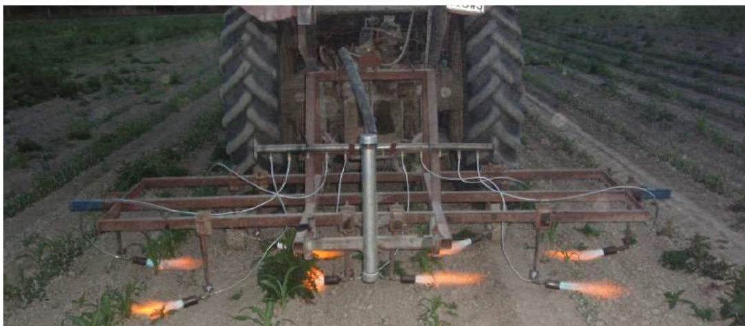
I Figure 30. Selective, intrarow flame weeder working in sweetcorn
