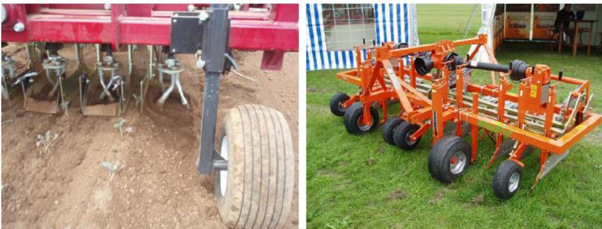
Figure 26. Vertical axis powered tine weeder
