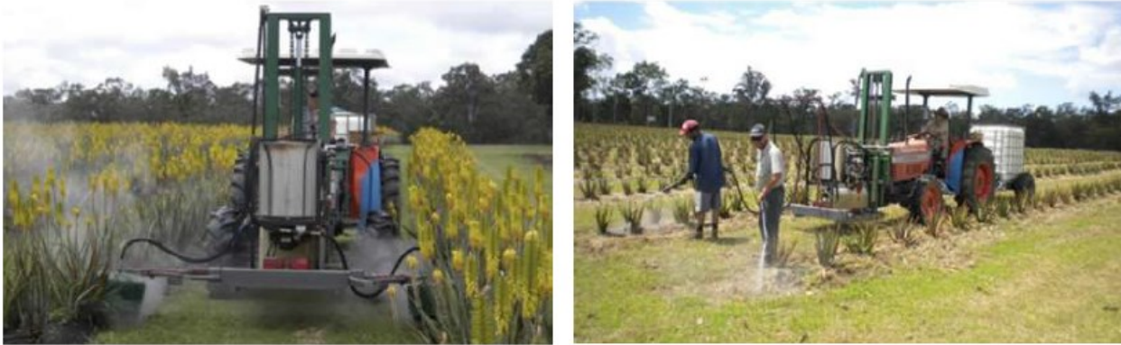
Figure 31. Intra-row steaming for weed management in perennial crop
